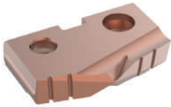
150° Structural Steel For material over 6mm thick and for reduced exit burr
