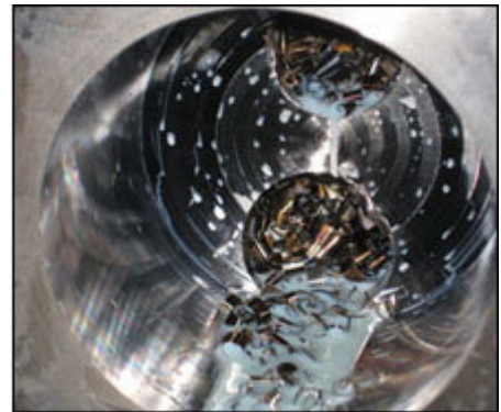
Allied's Opening Drill set to 5.01" (127.3 mm) went in over the top of the Revolution Drill and the two pre-existing holes in a 30 R c 4140 cylinder ram, double-cutting chips while handling a 0.620" (15.75-mm) offset cut with flood coolant.
