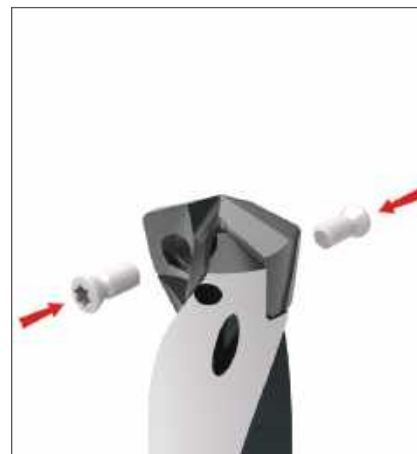
Step 3: Apply a generous amount of E-Z Break® (provided in the packaging) onto the supplied TORX® Plus screws.
