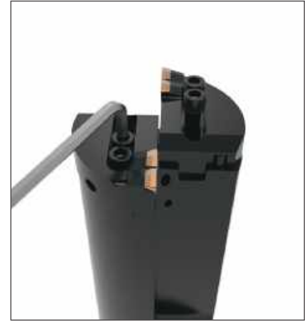
Step 3: Tighten the mounting screws on the cartridge to 15-19 N-m (11-14 ft-lbf).
