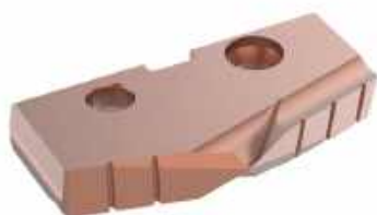
150° Structural Steel For material over 6 mm (7/16") thick and for reduced exit burr.
