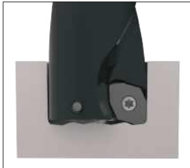
Periphery edge chip formation:
