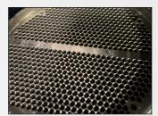
Knowing there had to be better options out there, the customer tested the **Superion Solid Carbide Drill** with HPS geometry and helical flutes that are ideal for drilling harder steels, high temp alloys, and stainless steel. Using the HPS geometry–designed to improve chip formation and reduce bell-mouth for longer drill depths—the customer gained consistent tool life.
