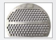
With 10,000 holes per stack plate assembly, the customer needed to produce a tight tolerance hole with a 32 Ra finish consistently through all five plates. The competition was running at 95 IPM (2413 mm/min) and only achieving a 63 Ra surface finish.
